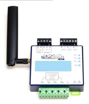
The MCCI® NerveCircuit™ Model 4811 is a complete integrated AC power measurement system for LoRaWAN® technology projects.
