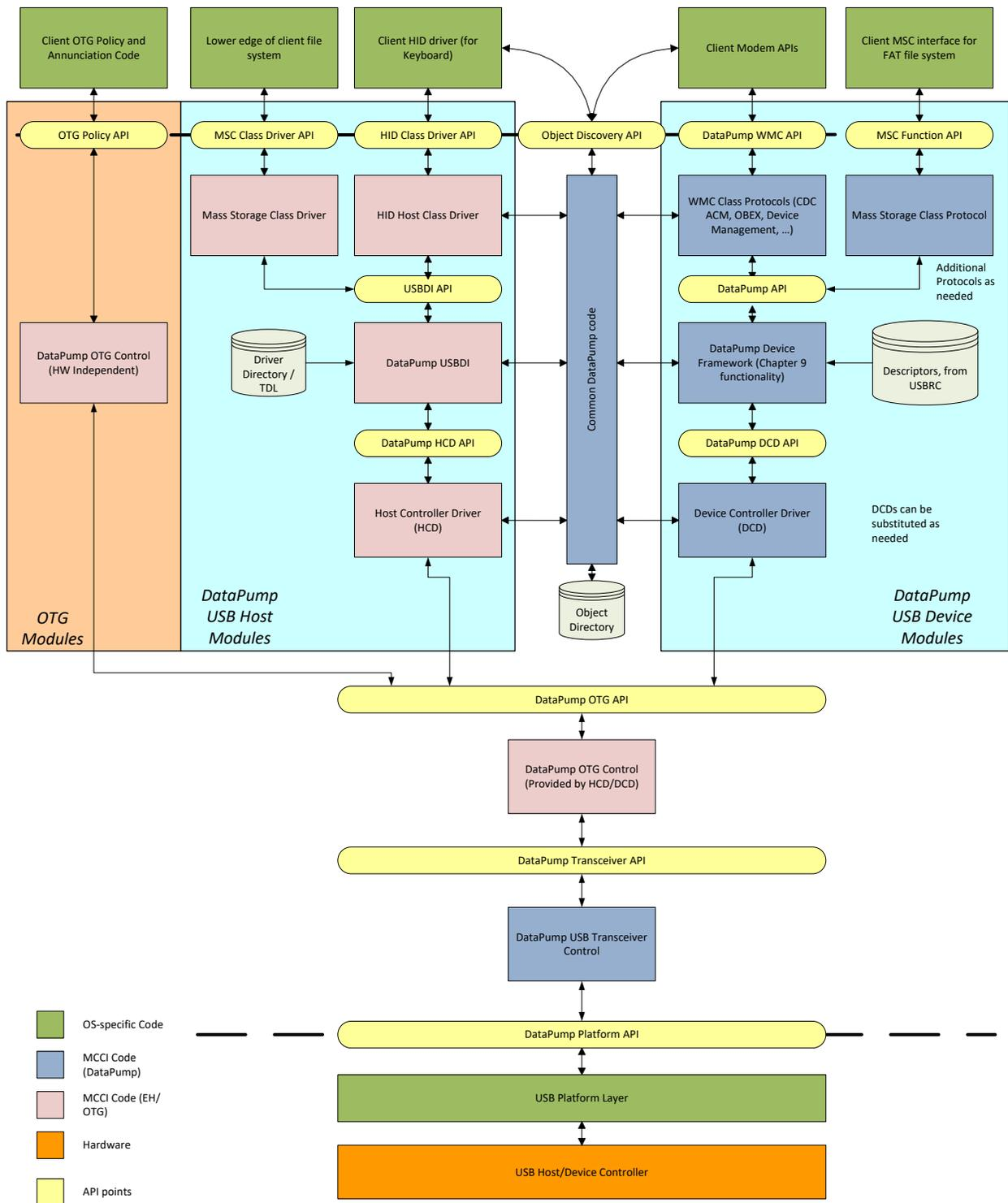
Figure 2. DataPump OTG Architecture
